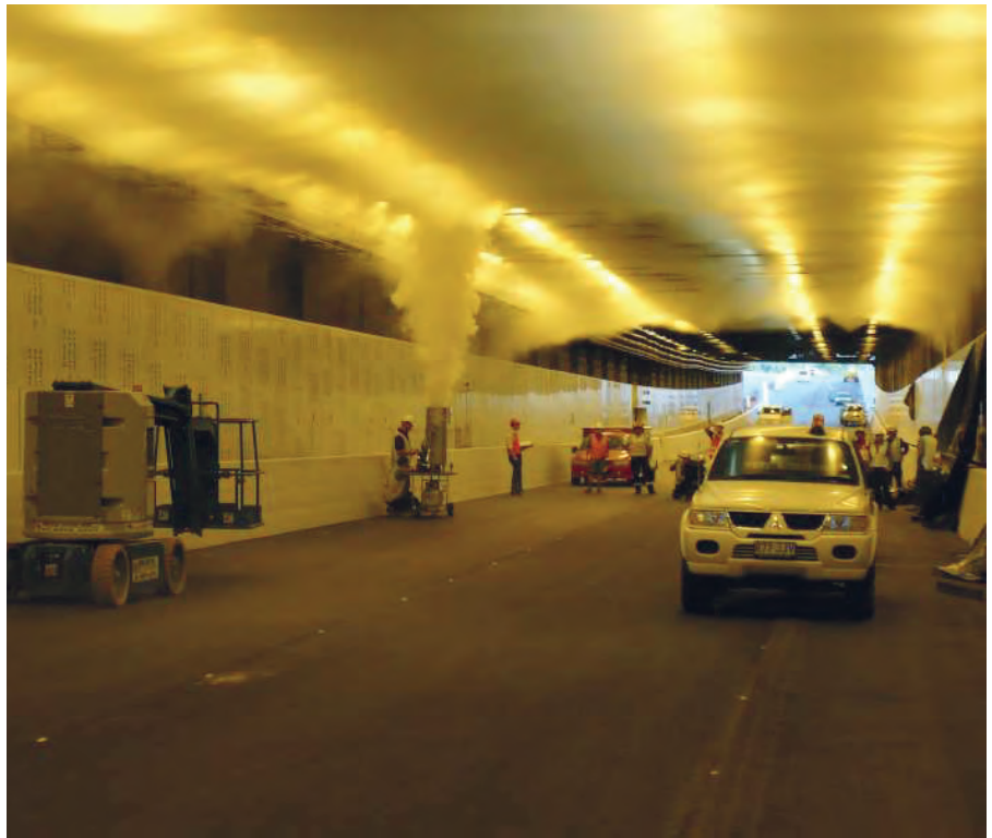
Smoke testing in the Tugun Bypass Tunnel, March 2008.
